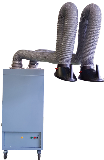
Image: An example of a two arm portable LEV extraction system (left) and a lightweight portable version suitable for on-gun extraction (right).
